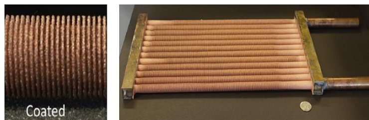
Fig. 1: Porous copper coated Capillary-assisted low-pressure evaporator (CALPE).
